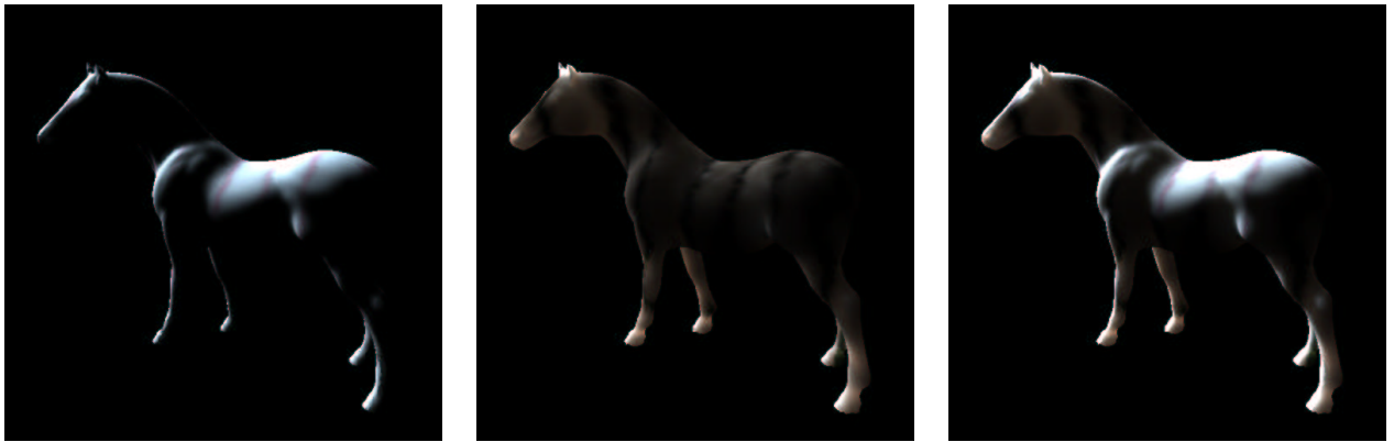
Figure 8. The textured horse model lit from the top left, parallel to the horse. The left image shows the local response, the middle the global response and the right image the combined result. Notice that different areas are illuminated due to local and global response.
