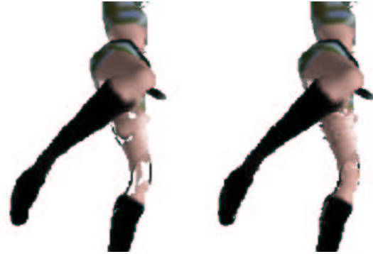
Figure 5: Influence of visibility maps in photo hull rendering. Eight reference views are used. Left: Without considering visibilities with respect to reference views, the black color from the raised foot participates in the color-consistency check. Therefore, some regions on the thigh of the other leg fail to be reconstructed. Right: These artifacts are removed when visibility maps are employed.
